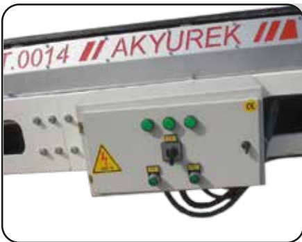
On Board Power Panel
